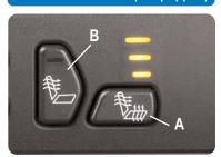
This feature allows you to heat the front seatbacks and seat cushions simultaneously or just the seatbacks. The controls are located on the driver and front passenger door panels.
